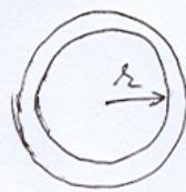
$$\frac{d}{dr} \left( KA \frac{dT}{dr} \right) + A Q = 0 \quad ; \quad \text{for } r_i < r < r_o$$
